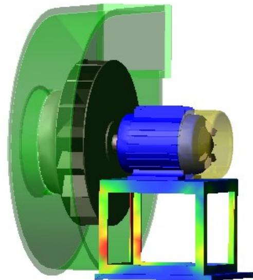
Machine vibrations are usually a disadvantageous phenomenon, that reduces the service life of structural elements as a result of impact and / or fatigue loads. Elements of a machine or structure subjected to static loads may have theoretically unlimited strength. Meanwhile, the variable load, with the amplitude corresponding to the value of the static load and the highly cyclical nature of the changes, will cause damage to the element in a finite time.
