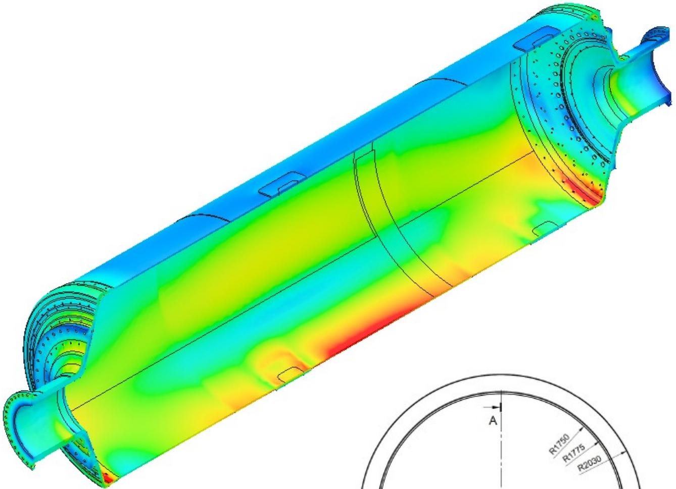
The aspects listed above are included in the finite element method using multi-node spatial three-dimensional elements (so-called **3D FEA**).
