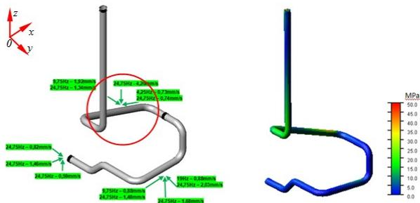
For example, the vibration parameters of selected pipeline cross-sections can be measured without contact (with a laser vibrometer), even when these places are not easily accessible. However, the determination of the stresses occurring in these sections in industrial conditions is much more difficult. Fortunately, they can be determined using numerical analysis - made on the basis of vibration measurements.
