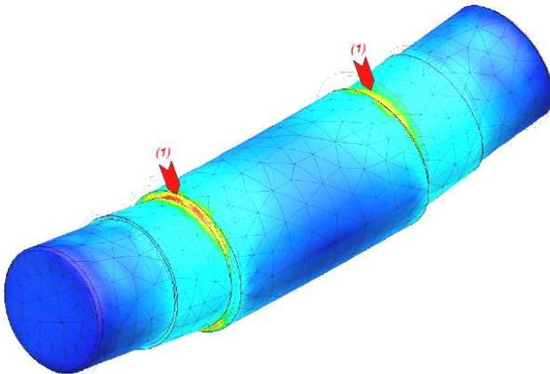
As part of the diagnostics of rotary drums, shell stress analyses are routinely carried out for objects considered as flexible. They are performed using the FEM method (Finite Element Method), most often in a simplified manner, based on the beam model, in accordance with the assumption that the stress state is decisively influenced by normal stresses caused by the bending moment.
